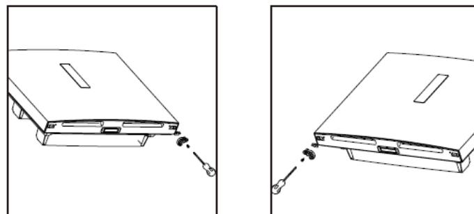
8. Make the middle hinge reverse the direction 180°C, then transfer it to the left property position. Make the middle hinge pin in the upper hole of the lower door, then tight the screws.
