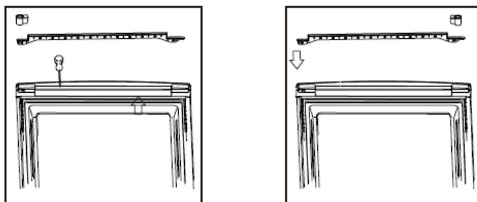
3. Unscrew from the middle hinge by cross screwriver, then take off the lower door.
