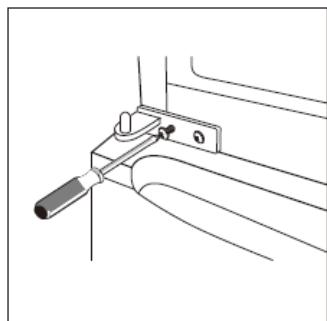
9. Install the upper door, fix the upper door hinge onto the cabinet and connect the wire.
