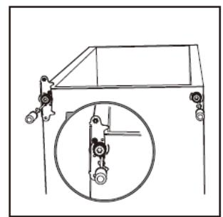
7. Unscrew right middle stopper with metal block from bottom of upper door. And then install left middle stopper and metal block in left side of bottom of upper door.
