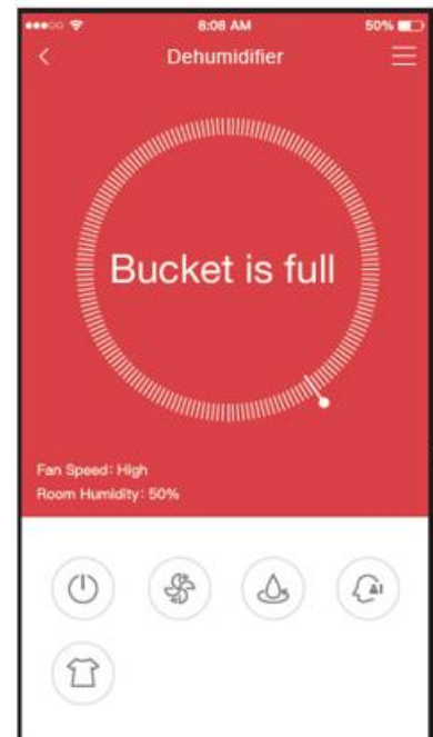
3. Make sure the Bucket is not full and place it in right position
