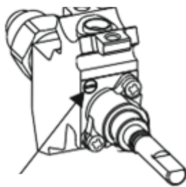
Surub de bypass
