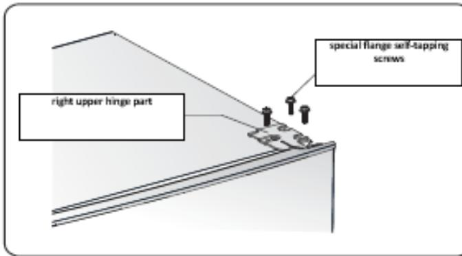
3. Remove the upper hinge axis, transfer it to reversed side and tighten security, then put it in a safe place.
