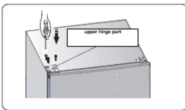
10. Install the screw hole on the top right corner of the appliance. Install the upper hinge cover (which is in the plastic bag) on the left corner. Pull the other upper hinge cover into the plastic bag.
