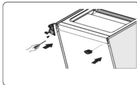
8. Transfer the door to the properly position, adjust the lower hinge part, make the hinge axis into the lower hole of the door.
