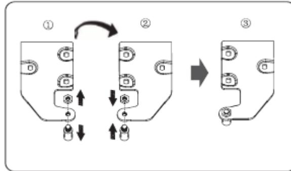
4. Remove the door from the lower hinge. NOTE: When removing the door, watch for washer(s) between the lower hinge and the bottom of the lower door that may stick to the door. Do not lose.
