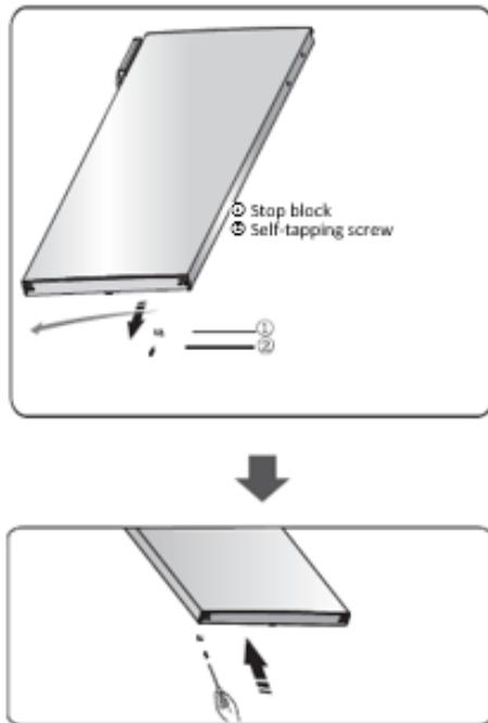
6. Lay the appliance on soft foam packaging or similar material. Remove both adjustable bottom feet parts, and the lower hinge part by unscrewing the special flange self-tapping screws.
