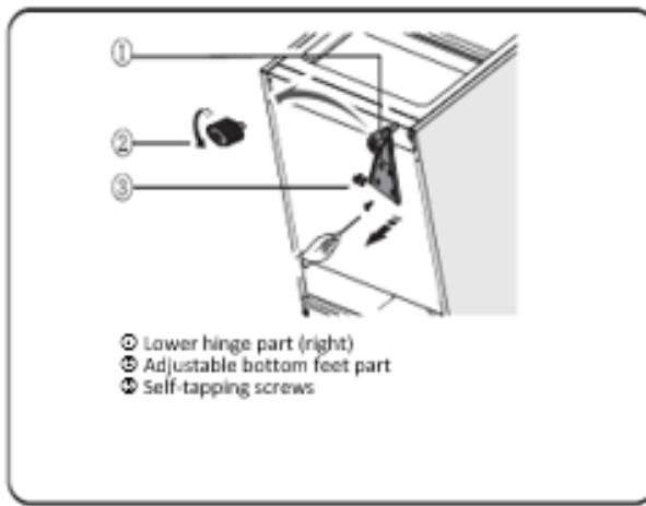
7. Replace the lower hinge part to the left side and fixing it with the special flange self-tapping screws. Replace the adjustable bottom feet parts to another side and fixing it.
