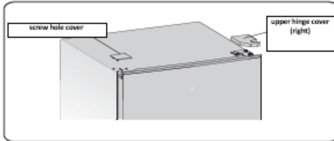
2. Unscrew the special flange self-tapping screws which are used for fixing the right upper hinge part by an 8 mm socket driver or a spanner (please support the upper door with your hand when doing it).
