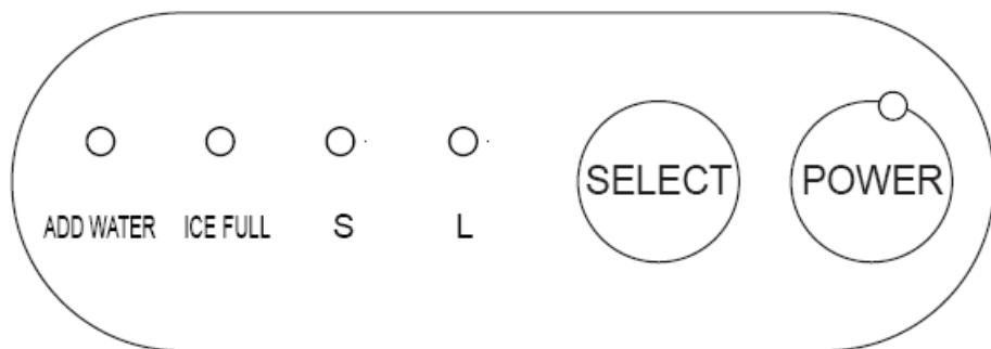
**POWER** - The indicator of POWER will flash after plugged in, and then the machine enters standby state. It will start to work by pressing POWER button, accompanying indicator lighting. During operation, pressing this button, the machine will return to standby state.
