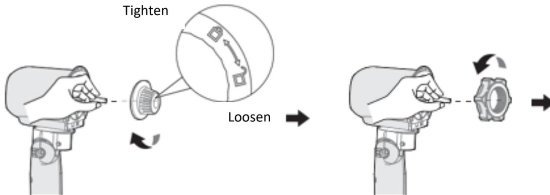
3.2. Hang the rear grille on the motor; rotate the grille lock nut clockwise to lock the rear grille
