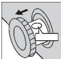
Rotate the drain dial 180 degree. This will let the water flow out in the tray.
