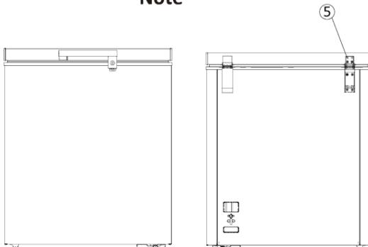
**NOTE:** if the lock ring failed to hold the lock when installing handle, please unscrew the round head screws (5) on the back of door and adjust the position of door upper and lower. Then drive the screw to fix the handle.
