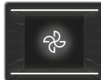
**Pizza Function:** The oven's thermostat and warning lights will switch on, and the ring, lower heating elements and fan will start operating. This function is ideal for baking food, such as pizza, evenly in a short time. While the fan evenly disperses the heat of the oven, the lower heating element ensures baking of the food.
