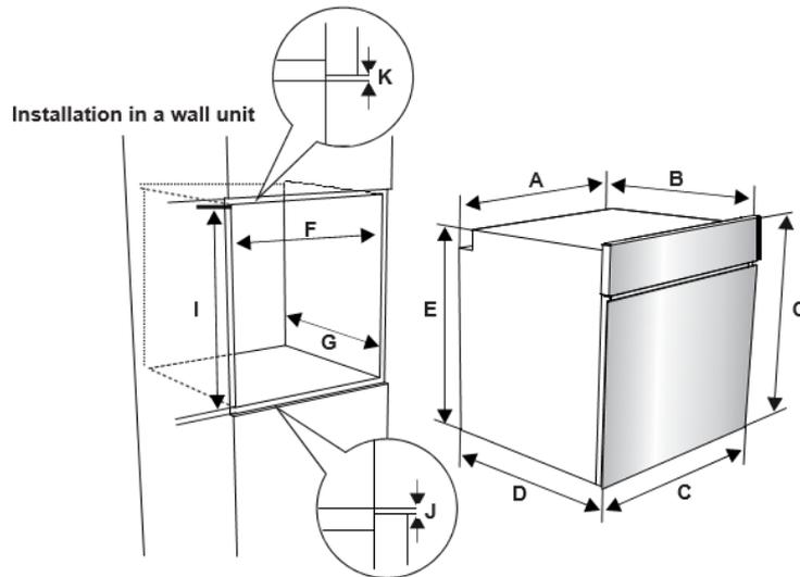
After making the electrical connections, insert the oven into the cabinet by pushing it forward. Open the oven door and insert 2 screws in the holes located on the oven frame. While the product frame touches the wooden surface of the cabinet, tighten the screws.
