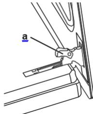
3. Close the door until it almost reaches the fully closed position and remove the door by pulling it towards you.
