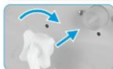
Connect the water supply hose to the water inlet valve and a water tap with cold water as indicated.
