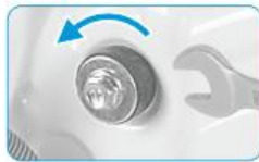
Loosen the 4 transport bolts with a spanner.
